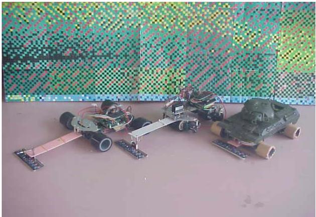
A photograph showing three custom-built microcontroller cars on a track. The cars are constructed from various materials, including metal and plastic, and are equipped with sensors and wheels. They are positioned on a track that has a white line on a dark surface. The background is a green and blue patterned wall. |
